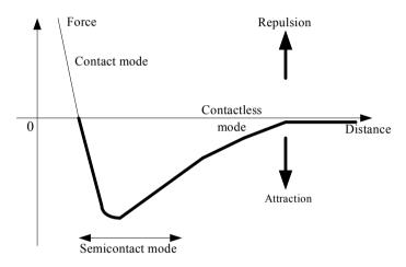
Fig. 6.3. The graph of the dependency of the Van der Waals force from the distance between the console and the sample surface
