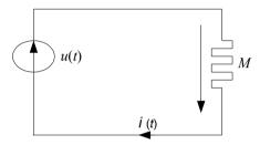
Fig. 4.1. Electrical circuit with the memristor
