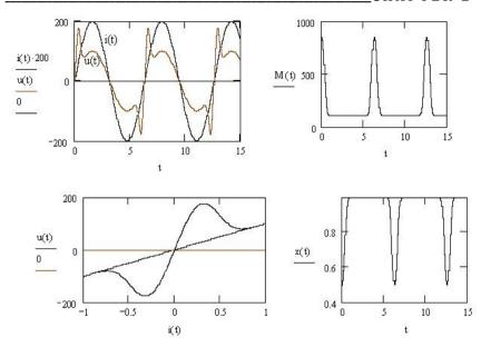
Fig. 2.4. Simulation results of the memristor described by the Nonlinear model Let's find the charge q(t) from the ratio
