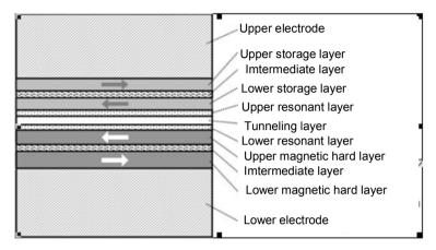
Fig. 7.20. Multilayer architecture of the MRAM cell
