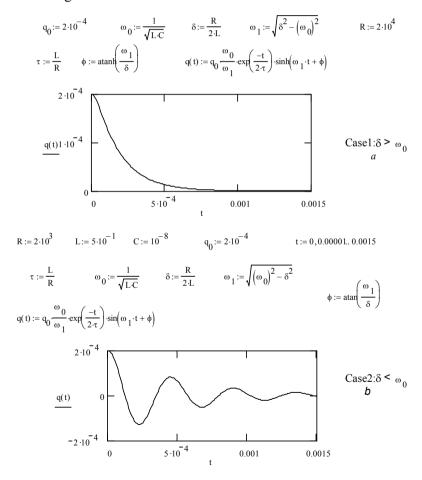
Fig. 4.12. The transients of the capacitor discharge
