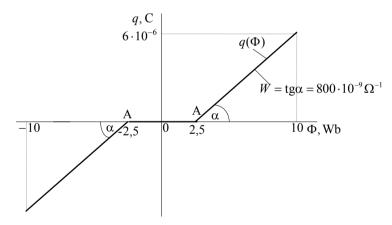
Fig. 5.4. Coulomb-weber characteristic of the memristor
