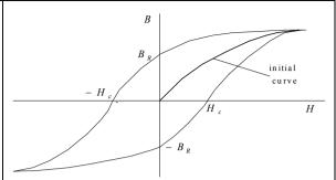
Fig. A1.4. The normal magnetization curve of the ferromagnetic
