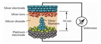
Fig. 5.13. Formation of the filament in the structure  $Ag/SiO_2/Pt$
