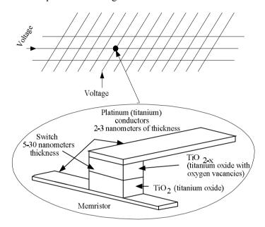
Fig. 1.6. Monolayer matrix of memristors
