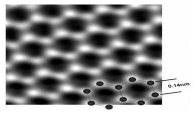
Fig. 7.23. Resolution of the scanning tunneling microscope
