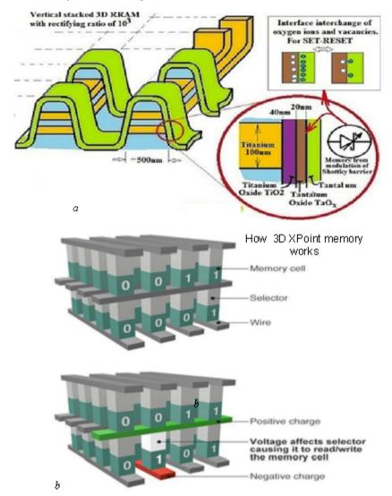
Fig. 7.7. The structure of the 3D memory of the ReRAM type
