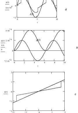
Fig. 5.3. Basic dependencies of the memristor controlled by the charge
