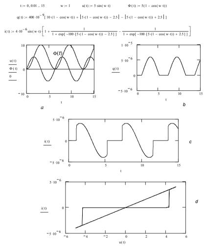
Fig. 5.6. Basic dependencies of the resistive switching
