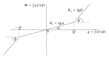
Fig. 5.1. The veber-coulomb characteristic of the memristor
