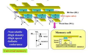
Fig. 7.17. The technology of manufacturing the memory matrix
