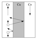
Fig. 7.9. Examples of the magnetic moments of the adjacent ferromagnetic layers
