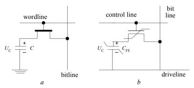
Fig. 7.32. Memory cell DRAM type (a) and 1T-1C FeRAM type (δ)
