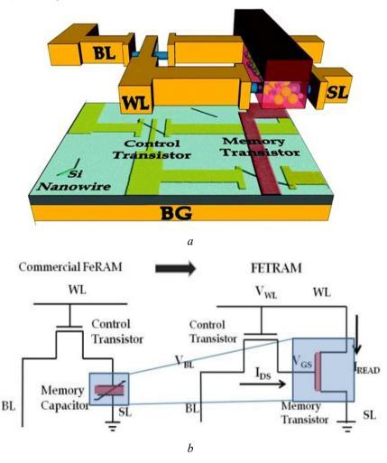
Fig. 7.34. (a) is the structure of the FeTRAM cell; (b) is the scheme of the cell
