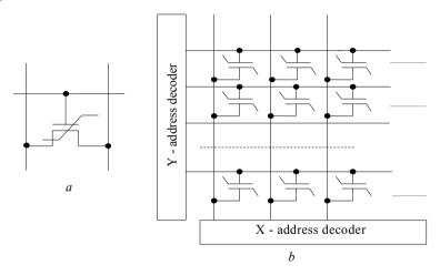
Fig. 7.31. (a) is the scheme of the 1TFeRAM cell type; (b) is the memory type 1SFeRAM (each cell contains one ferroelectric capacitor)
