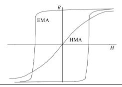
When the film thickness decreases to a few hundred Angstroms the magnetic film becomes the single-domain magnetic film with respect to its thickness. In this case a little time switching films  $(\sim 10^{-9} \text{ s})$  and high operation speed of the magnetic elements may be provided.
