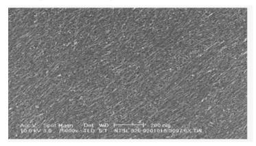
Fig. 7.50. The image of the film from the carbon nanotubes
