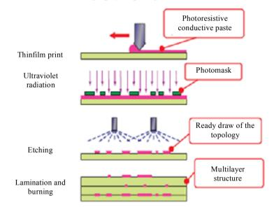
Fig. 6.6. The process of the photolithography
