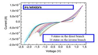
Fig. 5.15. The experimental current-voltage characteristics of the memristor with several intermediate states
