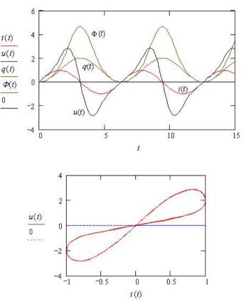
Fig. 1.9. Characteristics of the memristor controlled by charge
