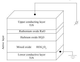
Fig. 6.11. The general structure of the memristor
