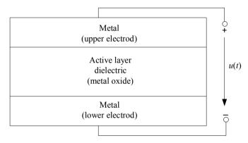
Fig. 5.7. MDM structure of the memristor
