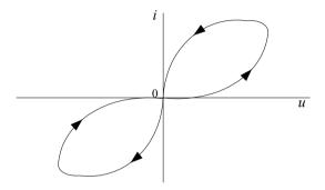
Fig. 1.22. The dependency i(u) of the memristor
