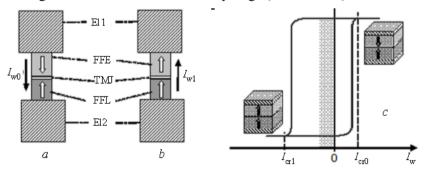
Fig. 7.54. The structural diagram of the memory cell
