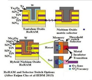
Fig. 7.4. Multilayer structures of the ReRAM memory cells
