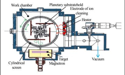
Fig. 6.13. Block diagram of the magnetron deposition plant
