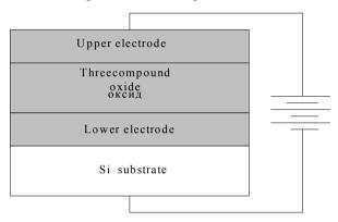
Fig. 6.8. MDM structure of the memristor
