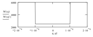
Fig. 5.2. The dependency of the memristance from the charge Then the charge passing through the memristor is equal to:
