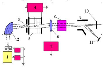
Fig. 6.10. A block diagram of an ion implantation
