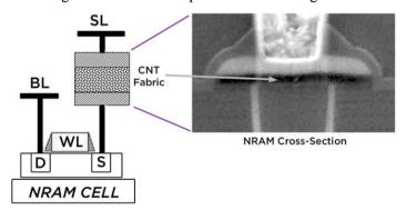
Fig. 7.53. The structure of the NRAM cell and the image of its cross-section
