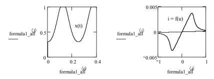
Fig. 2.9. Characteristics of the nonlinear model of the memristor with the window function  $f(x) = x - x^2$
