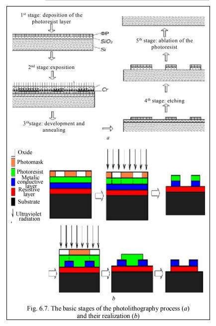
The principal difference of the photolithography from other types of the lithography is that the exposure is made by the visible or the ultraviolet light, whereas in other types of lithography the stream of ions, the electron stream, X-rays and other are used for this purposes.
