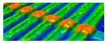
Fig. 5.10. The image of the memristors in the nodes of the matrix structure
