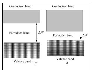
Fig. A1.5. Forbidden band: *a* is the dielectric; *b* is the semiconductor
