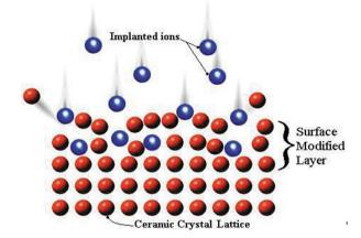
Fig. 6.9. The ion implantation process
