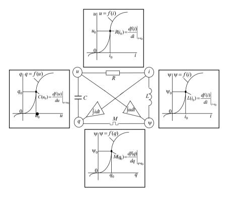
Fig. 1.7. Slope characteristics of fundamental elements
