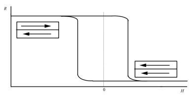
Fig. 7.14. The switching of the states in the MRAM cell
