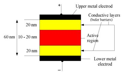
Fig. 7.37 The structure of the CeRAM memory cell
