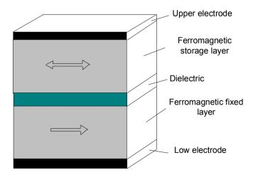
Fig. 7.13. The structure of the elementary cell
