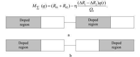
Fig. 4.4. Series connected memristors
