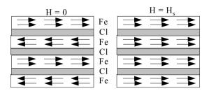
Fig. A3.1. Antiferromagnetic exchange coupling
