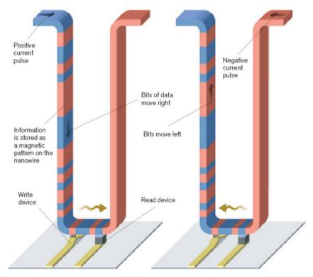
Fig. 7.45. Writing and reading operations used in the vertical location of the nanowires
