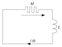
Fig. 4.8. Electric ML – circuit with the initial current
