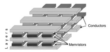
Fig.7.2. Forming 3D structure of the ReRAM memory
