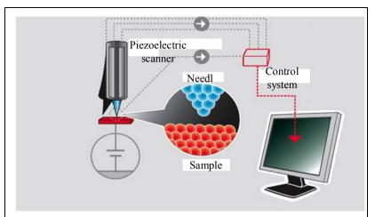
Fig. 7.22. The structure of the scanning tunneling microscope
