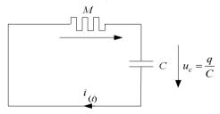
Fig. 4.5. The circuit of discharge of the capacitor
