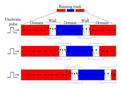
Fig. 7.42. Movement of the domain walls under the acting of the spin-polarized electric current
