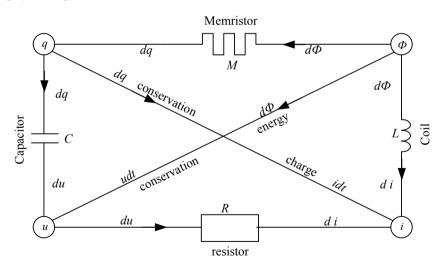
Fig. 1.2. Interconnection between the fundamental variables of electric circuits
