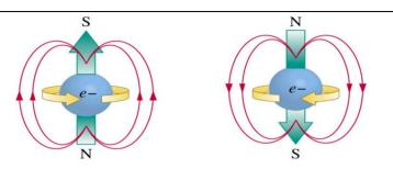
Fig. 7.12. Illustration of the spin-dependent tunneling effect
