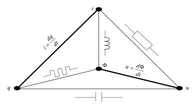
Fig. 1.3. Interconnection between the current, voltage, charge and magnetic flux
