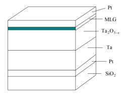
Fig. 7.5. Memory cell structure of the ReRAM type
