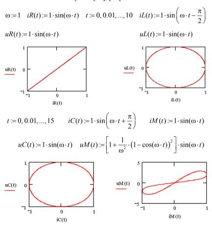
Fig. 1.16. Current-voltage characteristics of the fundamental elements
