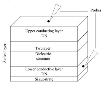
Fig. 6.18. Position of the probes with respect to the sample
