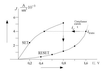
Fig. 7.36. Current-voltage characteristic of the CeRAM cell
