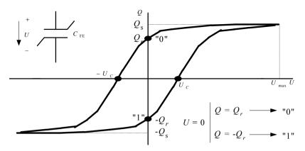
Fig. 7.30. The hysteresis loop of the ferroelectric capacitor
