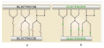
Fig. 7.52. The functioning diagram of the NRAM memory cell for the disconnection of the nanotubes (a) and their connection (b)
