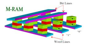
Magnetic tunnel junction is used to create the magnetic random access memory. The value of the MTJ transition resistance determines whether the resistance of the cell will read as "0" or "1", when the read current passes through the cell.
