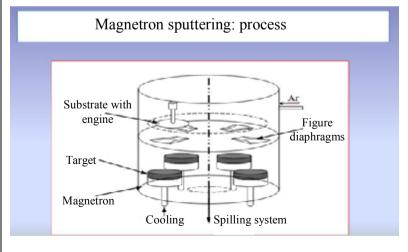
Fig. 6.12. Magnetron sputtering process
