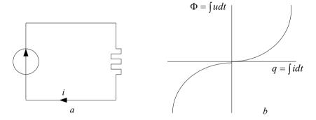
Fig. 1.8. Weber-Coulomb characteristic of the memristor
