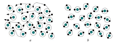
Fig. 7.41. The schematic difference between the states metal-insulator at the level of the nickel ions
