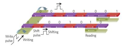
Fig. 7.46. Writing and reading operations used in the horizontal location of the nanowires
