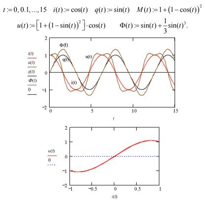
Fig. 1.13. Hysteresis loop degenerates into single-valued function
