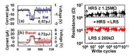
Fig. 7.51. The dependency of the consumed current from the applied voltage (*a*); the dependency of the memory cell resistance in the states with high resistance (HRS) and low resistance (LRS) from the number of the overwriting cycles (*b*)
