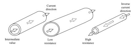
Fig. 1.17. Physical analogy of the memristor
