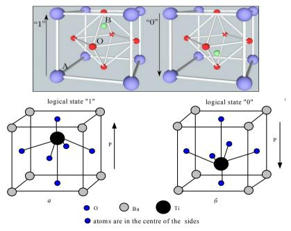
Fig. 7.28. The elementary cell of the barium titanate
