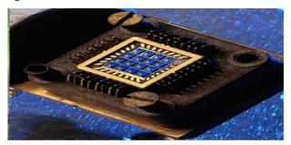
Fig. A3.3. The chip with the spin transistors
