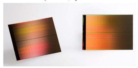
Fig. 7.8. Nonvolatile memory 3D X Point of the ReRAM type
