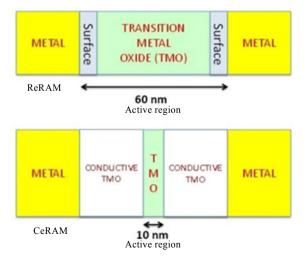
Fig. 7.38. Structures of the ReRAM and CeRAM
