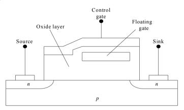
Fig. 7.1. The scheme of the field effect transistor with the floating gate
