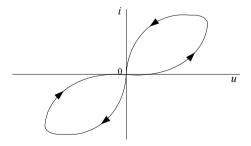
Fig.1.1. Current-voltage characteristic of a memristor
