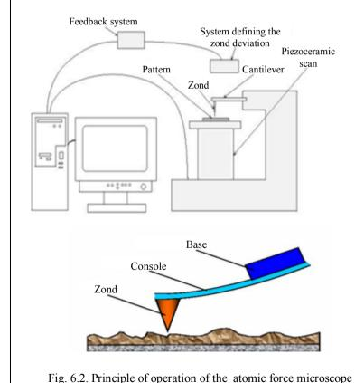
The force acting on the probe from the surface leads to the bend of the console. The forces acting between the probe and the sample represent, primarily the long-distance Van der Waals forces (intermolecular forces, which are based on the electrostatic interaction of the dipoles), which at first are the forces of attraction, and with the further rapprochement these forces are transformed into the repulsive forces, Fig. 6.3.
